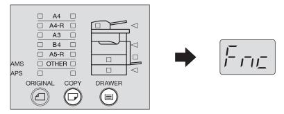
Press the [DRAWER] button several times until the lamp of the bypass tray is lit.
